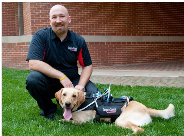
"We're developing a platform for sensors that is designed to be plug-and-play, allowing emergency responders to further customize the harness," Bozkurt says. "For example, if there's the possibility of a natural gas leak, you could attach a natural gas sensor. Or if there's the possibility of radiation, you could attach a Geiger counter." Using wireless communications, the sensors can be monitored remotely at a command center or by dog handlers on a handheld device nearby.
